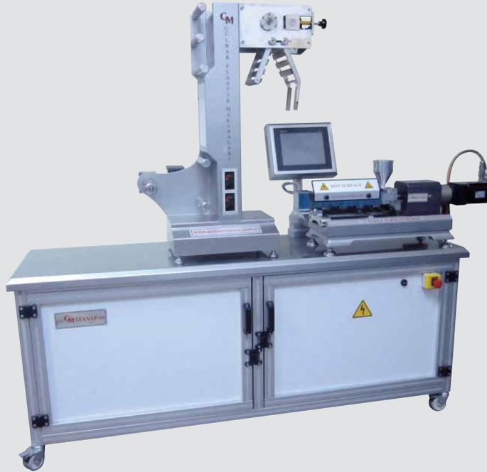
16 mm single screw extruder has different barrels like 24 L/D - 30 L/D - 35 L/D. It's possible to interchangeable barrel length between 24 L/D to 35 L/D depending to the customer needs . Barrel consist of seven parts and all these parts are resistant to high temperatures. To have a better mixture and a better dispersion all zones heaters can be controlled at different temperatures at the same time.
