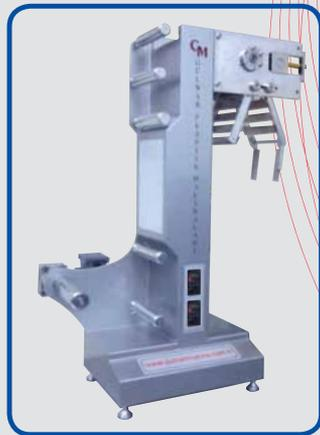
The film blowing unit simultaneously blows up, cools, takes off, and winds up your extruded blown films. The bubble diameter and film thickness can be adjusted precisely.
