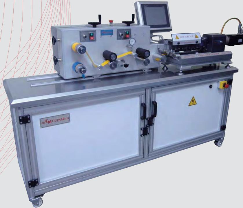
16 mm single screw extruder has different barrels like 24 L/D - 30 L/D - 35 L/D. It's possible to interchangeable barrel length between 24 L/D to 35 L/D depending to the customer needs . Barrel consist of seven parts and all these parts are resistant to high temperatures. To have a better mixture and a better dispersion all zones heaters can be controlled at different temperatures at the same time.
