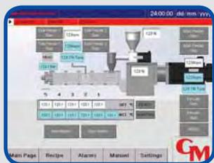
With very friendly user control software and 10'' touch screen the control of rotational speed of feeder and screw, the set value of heaters can be adjusted very easily. In same time the Head pressure and the zone temperature values can be read from same screen. Also operator is able to create unlimited new methods for different polymers, call and load them in control panel as needed.
