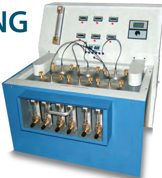
medium and enters the cell through a diffuser nozzle for even air flow distribution. For safety, the apparatus is fitted with an over temperature thermostat which switches off the apparatus if it over heats.
