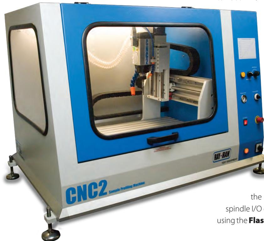
spindle speeds can be set within the G-Code program file and spindle on/off functions selected using specified M-codes. High quality custom made single flute tungsten carbide cutters ensure a superior finish on any machined sample.
